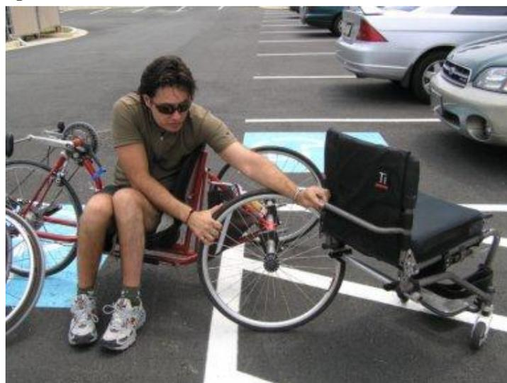
3. After you have it behind the handcycle, you will need to line up the WB's with either the anti-tipper slots or the end-tubes and slide the long bolts of the WB into those slots. This is when it
